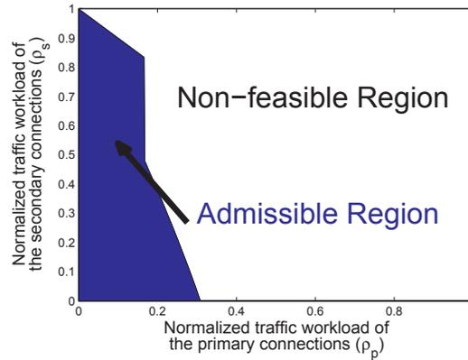
Fig. 8. Admissible region for the normalized traffic workloads  $(\rho_p, \rho_s)$ , where the average cumulative delay constraint can be satisfied when  $t_s = 0$  (slot),  $\mathbf{E}[X_p] = 20$  (slots/arrival) and  $\mathbf{E}[X_s] = 10$  (slots/arrival).
