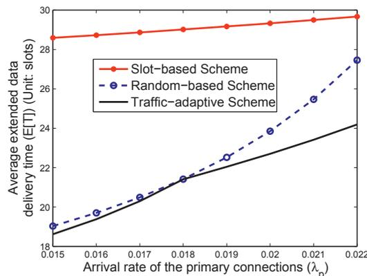
Fig. 9. Comparison of average extended data delivery time for different target channel selection sequences.
