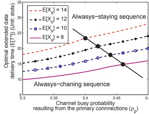
Fig. 7. Effects of secondary connections' service time  $\mathbf{E}[X_s]$  on the cross-point for the traffic-adaptive channel selection approach, where  $t_s = 1$  (slot),  $\mathbf{E}[X_p] = 20$  (slots/arrival), and  $\lambda_s = 0.01$  (arrivals/slot).
