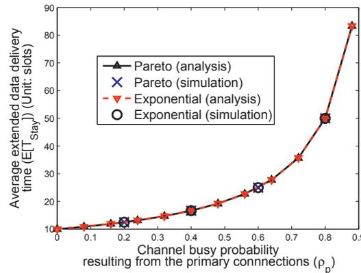
Fig. 5. Effects of Pareto and exponential service time distributions for primary connections on the extended data delivery time ( $\mathbf{E}[T_{stay}]$ ) of the secondary connections when the **always-staying** spectrum handoff sequence is adopted, where  $t_s = 1$  (slot),  $\lambda_s = 0.01$  (arrivals/slot),  $\mathbf{E}[X_s] = 10$  (slots/arrival), and  $\mathbf{E}[X_p] = 20$  (slots/arrival).
