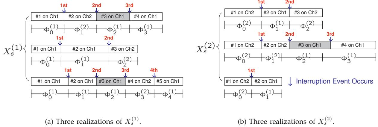
Fig. 3. Illustration of the physical meaning of random variable  $\Phi_i^{(k)}$ . For example,  $\Phi_2^{(1)}$  is one of the third segments (gray areas) of the first and the third secondary connections in (a) as well as the second secondary connection in (b). Note that the third secondary connection in (b) does not have the third segment because it is interrupted only once.
