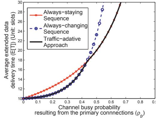
Fig. 6. Comparison of the extended data delivery time for the always-staying and always-changing spectrum handoff sequences as well as the traffic-adaptive channel selection approach, where  $t_s = 1$  (slot),  $\lambda_s = 0.01$  (arrivals/slot),  $\mathbf{E}[X_p] = 20$  (slots/arrival), and  $\mathbf{E}[X_s] = 10$  (slots/arrival).
