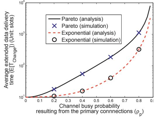
Fig. 4. Effects of Pareto and exponential service time distributions for primary connections on the extended data delivery time ( $\mathbf{E}[T_{change}]$ ) of the secondary connections when the **always-changing** spectrum handoff sequence is adopted, where  $t_s = 1$  (slot),  $\lambda_s = 0.01$  (arrivals/slot),  $\mathbf{E}[X_s] = 10$  (slots/arrival), and  $\mathbf{E}[X_p] = 20$  (slots/arrival).
