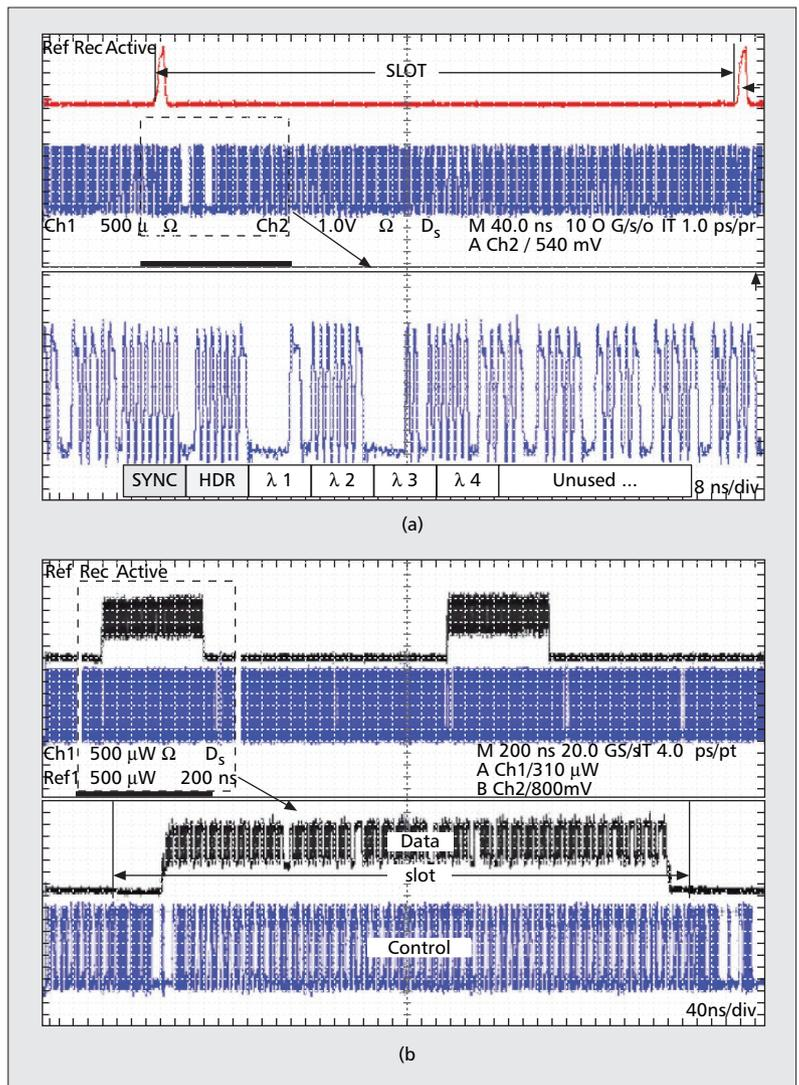
■ Figure 4. Synchronization of control and data channels: a) control channel slot; b) synchronized data and control slots.
