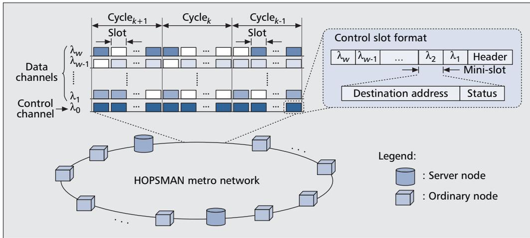
■ **Figure 1.** General architecture of the HOPSMAN network testbed.
