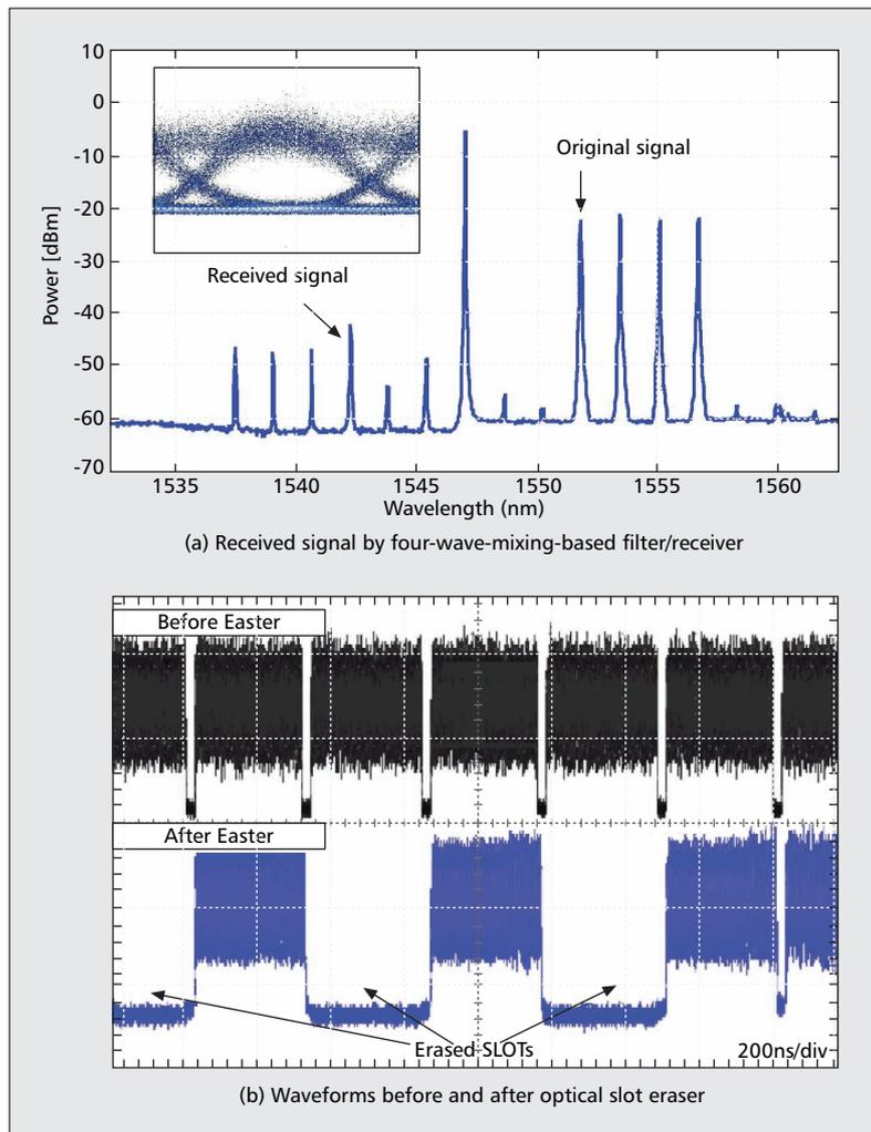
**Figure 5.** Experimental results with fast optical devices: a) received signal by FWM-based filter/receiver; b) experimental results with fast optical devices.
