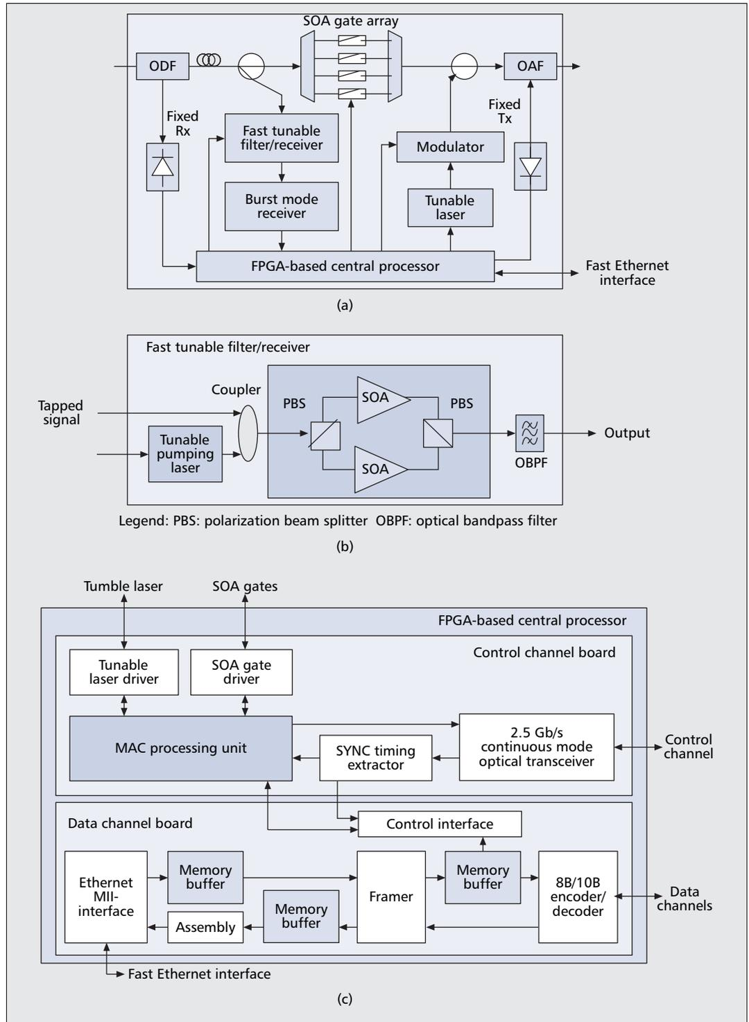
■ **Figure 3.** Hardware implementation of the HOPSMAN testbed system: a) experimental node setup (S-node); b) four-wave-mixing-based fast tunable filter/receiver; c) FPGA-based central processor.
