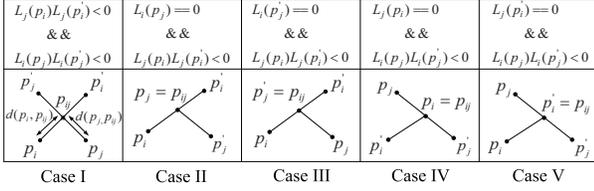
Fig. 1. Possible intersection (collision) cases generated by moving paths of any two sensors  $s_i$  and  $s_j$ , where  $p_i$  ( $p_j$ ) denotes the original position of  $s_i$  ( $s_j$ ) and  $p'_i$  ( $p'_j$ ) indicates the physical movement destination for sensor  $s_i$  ( $s_j$ ).
