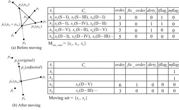
Fig. 2. Every sensor  $s_i$  in the potential moving set  $M_{min\_order}$  should be analyzed by identifying its intersection (collision) relationship with each member in  $C_i$ , in which intersection cases D-II, D-IV, S-I, S-II, S-III, S-IV, and S-V require further consideration/processing, before including  $s_i$  into the moving set (allowed to move in the current round).
