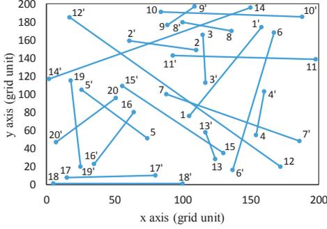
Fig. 3. Random path configuration in a monitored  $200 \times 200$  area with sensors population up to 20 (here  $i$  represents the departure position of sensor  $s_i$  whereas  $i'$  indicates the destination (goal) position of  $s_i$ ).
