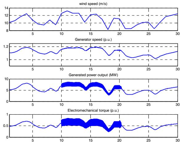
Fig. 14. Simulation Results of Wind Speed (m/s), Generator Speed (p.u.), Generated Power Output (MW) and Electromechanical Torque (p.u.)
