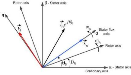
Fig. 4. Vector Diagram in a Field Oriented Control
