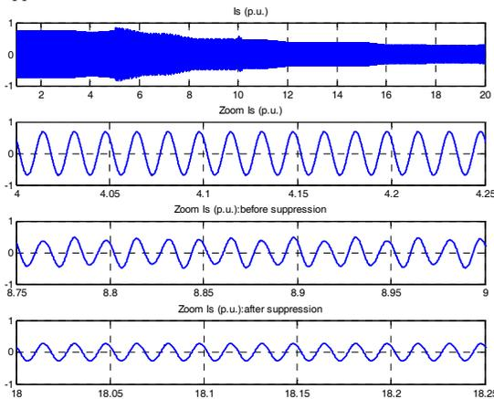
Fig. 12. Simulation Results of Generated Current Output (p.u.) and Zoomed Current Output (p.u.) Before and After Suppression
