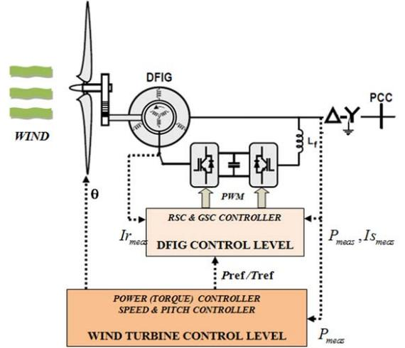
Fig. 3 Configuration of a DFIG wind turbine
