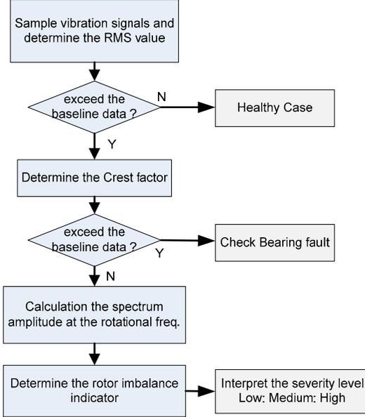
Fig. 2. Mechanical vibration analysis for wind turbine monitoring system
