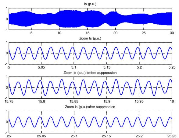
Fig. 16. Simulation Results of Generated Current Output (p.u.) and Zoomed Versions of Current Output (p.u.): Before and After Suppression
