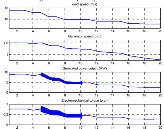
Fig. 10. Simulation Results of Wind Speed (m/s), Generator Speed (p.u.), Generated Power Output (MW) and Electromechanical Torque (p.u.)
