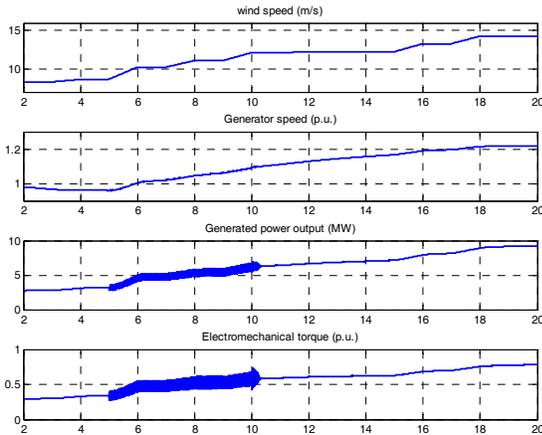
Fig. 7. Simulation Results of Wind Speed (m/s), Generator Speed (p.u.), Generated Power Output (MW) and Electromechanical Torque (p.u.) responded on Wind Ramp up Event
