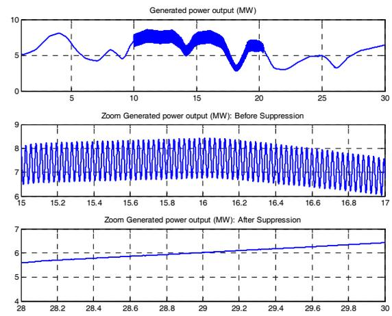
Fig. 15. Simulation Results of Generated Power Output (MW): Before and After Suppression
