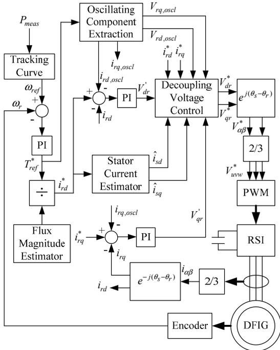
Fig. 5. Proposed control structure of the rotor side inverter controller
