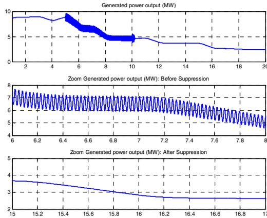
Fig. 11. Simulation Results of Generated Power Output (MW): Before and After Suppression
