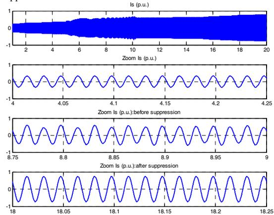
Fig. 8 Simulation Results of Generated Current Output (p.u.) and Zoomed Versions of Current Output (p.u.): Before and After Suppression
