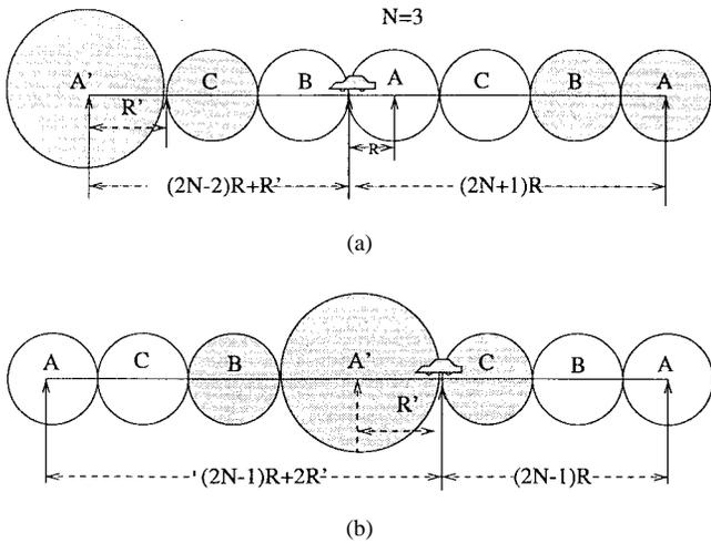
Fig. 2. A one-dimensional mixed-cell architecture, where: (a) indicates the macro-cell imposes the interference on the micro-cells and (b) shows the opposite situation.
