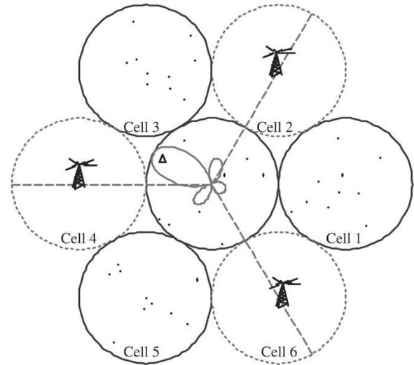
(a) : Beamforming with beam-steering technique
