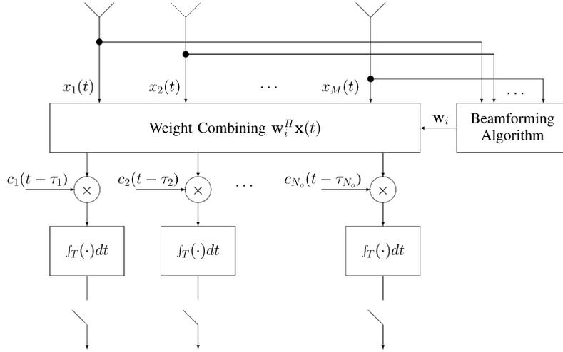
Fig. 3. Receiver block diagram with antenna beamformers.
