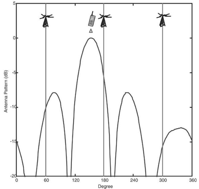
(b) : Antenna pattern with beam-steering technique
