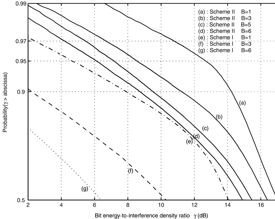
Fig. 8. Uplink performance comparison of Schemes I and II with different numbers of cells generating the opposite-direction interference (denoted as  $B$ ). Note that, in this case, the number of antenna elements is equal to nine.
