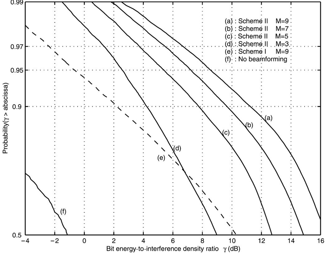
Fig. 7. Uplink performance comparison of Schemes I and II with different numbers of antenna elements (denoted as  $M$ ). Note that, in this case, the number of cells generating the opposite-direction interference is equal to three.
