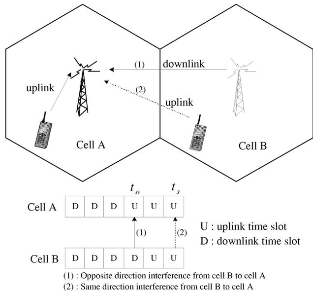
Fig. 1. Opposite-direction interference in the TDD/CDMA system.
