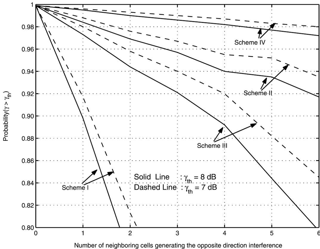
Fig. 10. Performance comparison of four beamforming schemes with different numbers of cells generating the opposite-direction interference, where an antenna array with nine elements is deployed at base stations.
