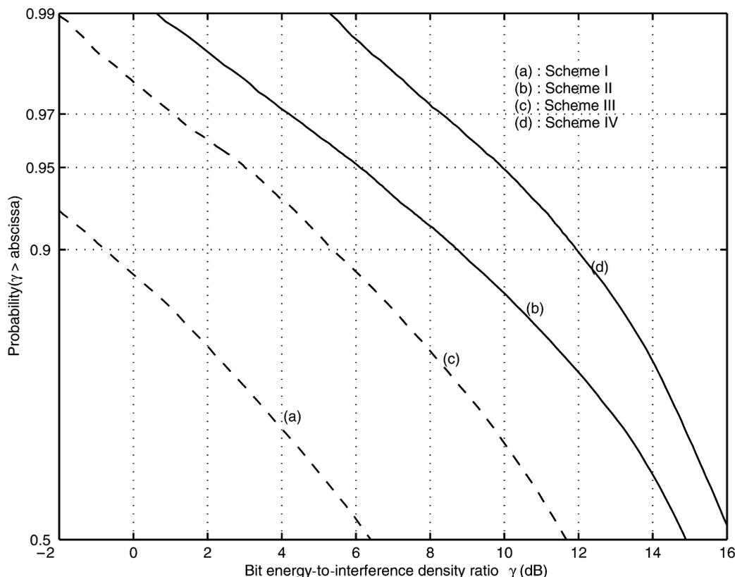
Fig. 9. Performance improvements by implementing downlink transmitting beamformer in the surrounding base stations, where the number of cells generating the opposite-direction interference equal to six and the number of antenna elements equal to nine.
