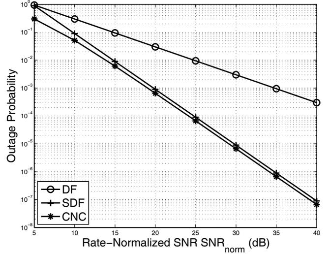
Fig. 3. Comparison of outage probability for decode-and-forward (DF), selection decode-and-forward (SDF), and cooperative network coding (CNC) protocol when the data rate  $R$  is equal to 1 bps/Hz.
