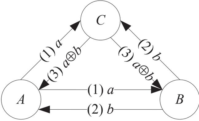
Fig. 1. System model and the CNC protocol, where phase (1):  $A$  sends  $a$  to  $B$  and  $C$ ; phase (2):  $B$  sends  $b$  to  $A$  and  $C$ ; phase (3):  $C$  broadcasts  $a \oplus b$  to  $A$  and  $B$ .
