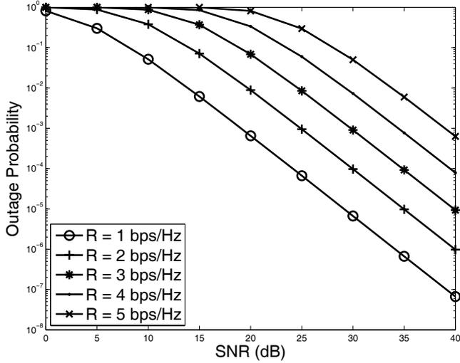
Fig. 2. Outage probability for the cooperative network coding (CNC) protocol when the data rate  $R$  is equal to 1, 2, 3, 4, 5 bps/Hz.
