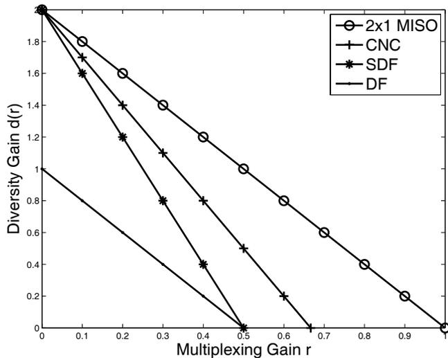
Fig. 4. Comparison of diversity-multiplexing tradeoff the  $2 \times 1$  multiple-input single-output (MISO) system, cooperative network coding (CNC), selection decode-and-forward (SDF), and decode-and-forward (DF).
