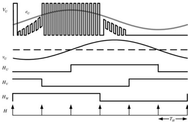
Figure 4 Illustrated waveforms for BEDC-I with FUPWM
