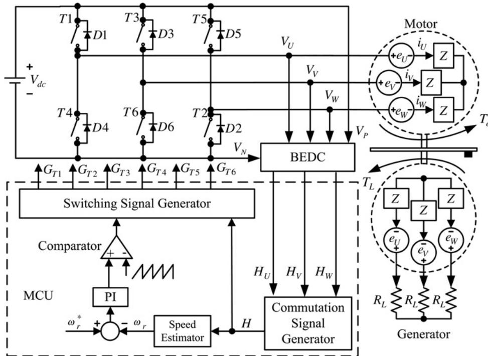
Figure 1 Configuration of sensorless control with 120° SWPWM
